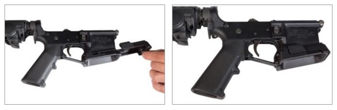
Install the screws through the ears of the bottom piece into the top piece. Alternate tightening the screws to ensure the magwell is positioned correctly and properly installed. DO NOT EXCEED 15 IN-LBS OF TORQUE.
