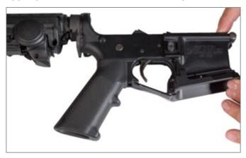
4. Slide the top piece of the magwell extension onto the bottom piece and lower receiver (from front to rear).
